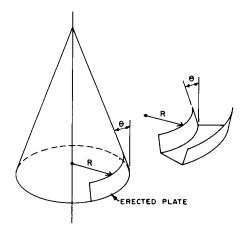
CONICAL DEVELOPMENT OF INCLINED WEB
